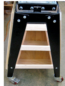
End Storage Compartment Installed
