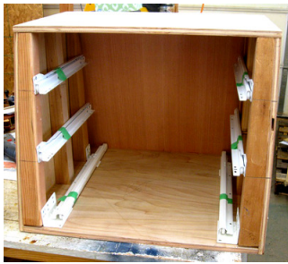
Drawer Box -- Front View Note: Tapered Side Furring Strips
