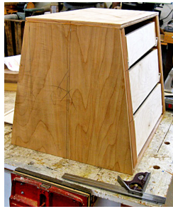
Drawer Box -- End View Note: Slanted Drawer Faces
